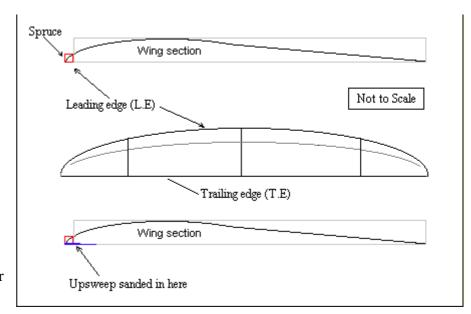
A Spruce leading edge will strengthen the wing and help prevent LE damage.
